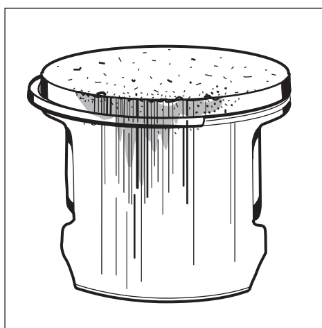
Exhaust side damaged by a broken piston ring. The piston ring parts damage the top section and cause score marks.
