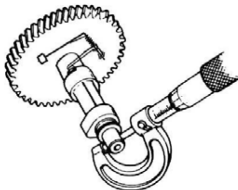
Figure 4-45: Measure Camshaft Journal
