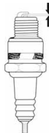
Figure 3-4: Verify Spark Plug Gap
