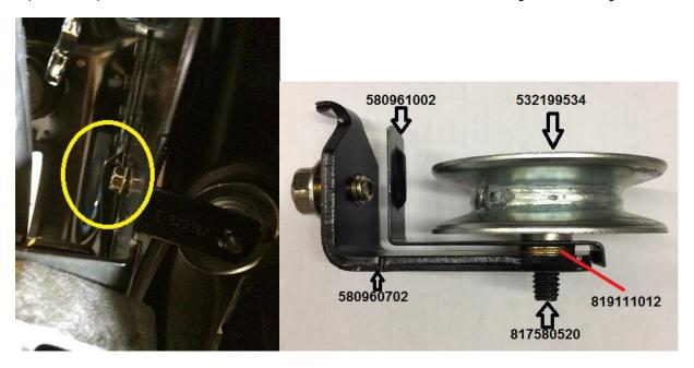
**Step 4**. When replacing bracket, ensure tang on bracket is locked into chassis. Tighten bolt and ensure belt is between keeper and pulley.
