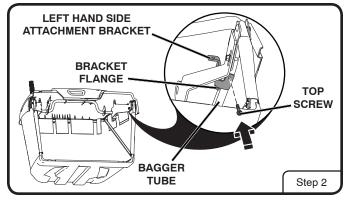
**Step 2:** Install side attachment bracket onto left hand side using top screw previously removed as shown in illustration. Ensure bracket flange is flush against bagger tube. Torque top screw to 48 - 72 In. Lbs. (5.4 - 8.1 Nm). Repeat steps 1 and 2 for the right hand side attachment bracket.
