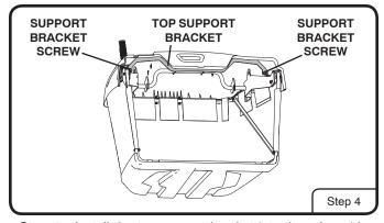
**Step 4:** Install the top support bracket into the other side attachment bracket using the remaining support bracket screw. Torque the second support bracket screw to 15 - 20 Ft. Lbs (20 - 27.1 Nm). Once completed, torque the first support bracket screw to 15 - 20 Ft. Lbs (20 - 27.1 Nm).
