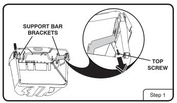
**Step 1:** Remove top screw from the left hand side of the front of the bagger assembly. Save top screw for future use.
