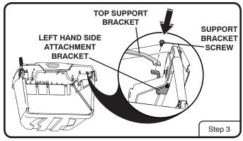
**Step 3:** Install and hand-tighten top support bracket into one of the side attachment brackets using one of the support bracket screws supplied with kit.
