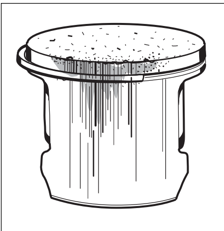
Exhaust side damaged by a broken piston ring. The piston ring parts damage the top section and cause score marks.
