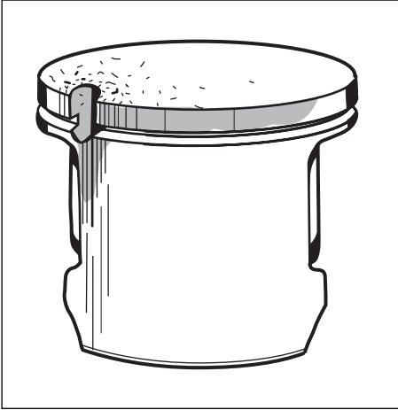
The guide pin for the piston ring has been pushed up through the top of piston.
