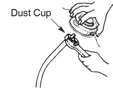
2. Remove trimmer head by turning counterclockwise (looking from bottom of unit).
