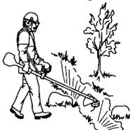
4. Switch off the engine before moving to another area. Fit the transport guard before carrying or transporting the equipment any distance.
