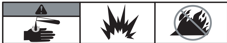
Battery acid is corrosive, explosive and flammable
