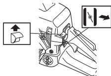
**Startgass:** Kombinert choke/startgass-stilling oppnås når hendelen stilles i choke-stilling.
