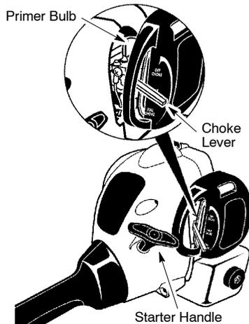
6. Pull starter rope handle sharply until engine sounds as if it is trying to start, but do not pull rope more than 6 times.
